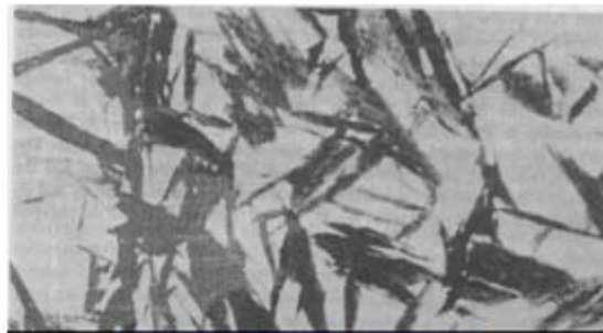
Bainite formed at 278°C
