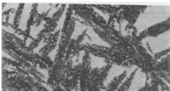
Bainite formed at 348°C
